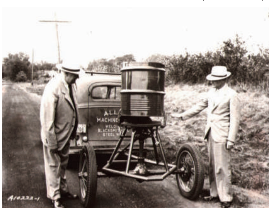
An applicator for granular insecticide or poisoned bait. C.J. Drake (left) and C.H. Richardson. October 3, 1938.
